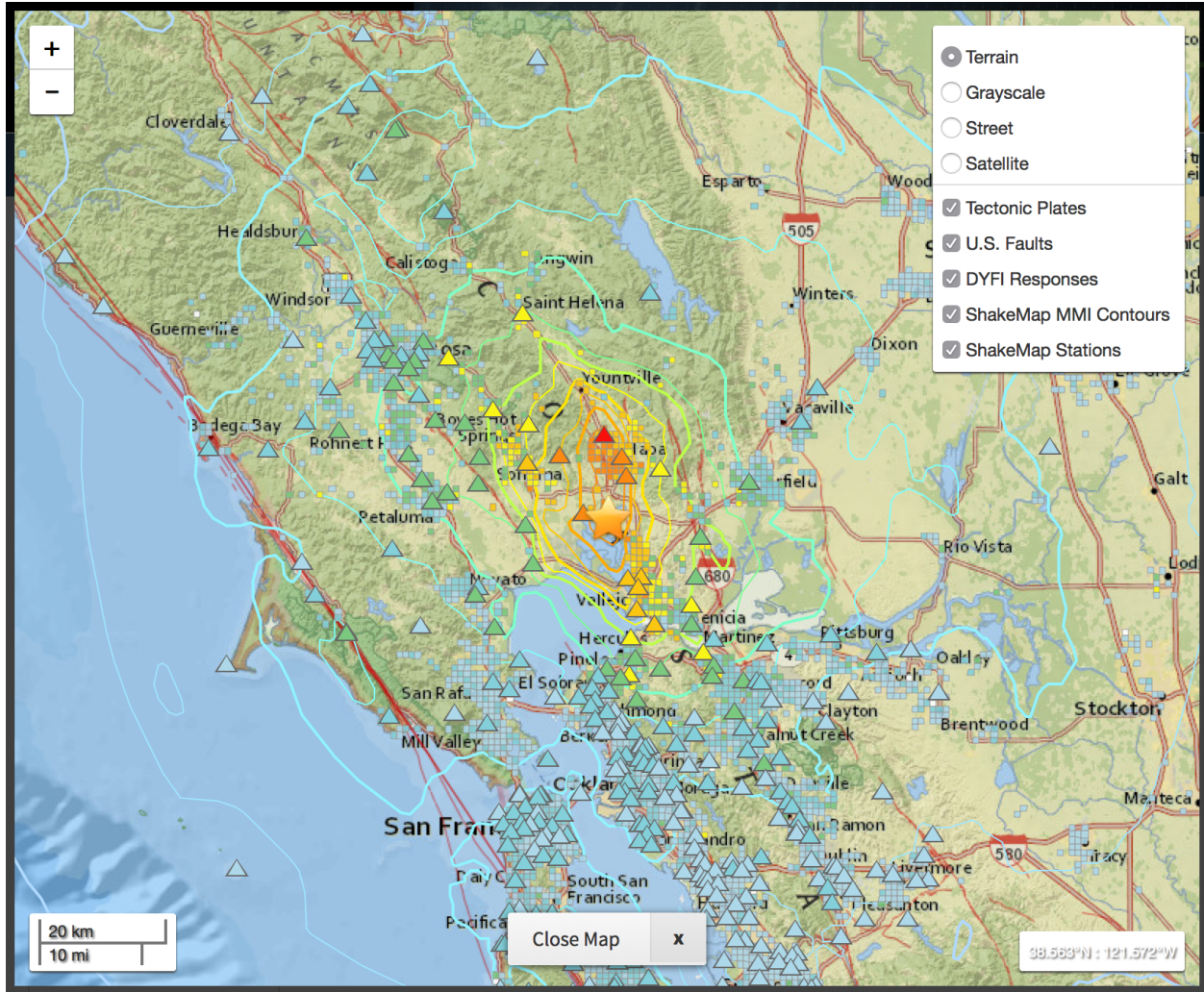
Fig. 1.25: Interactive ShakeMap for the 2014 M6.0 American Canyon, CA earthquake. On the interactive map, reported (DYFI) intensities are geocoded and represented with squares depicting the 1km grid area they occupy. Reported Intensities are color-coded according to their intensity value, either as observed or as converted by Wald et al. (1999b) .
