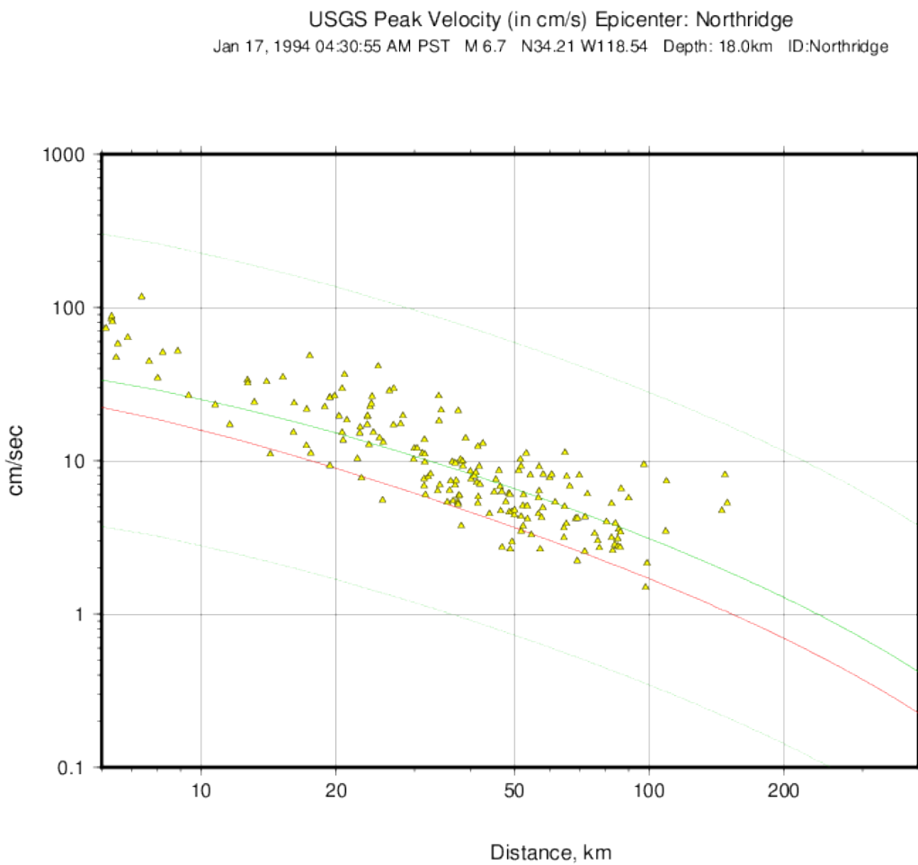
Fig. 1.12: Plot of Northridge earthquake PGVs as a function of distance. The triangles show recorded ground motions; the red line shows the unbiased Boore and Atkinson (2008) (BA08) GMPE; the dark green lines show BA08 following the bias correction described in the text; the faint green lines show the bias-adjusted GMPE \pm three standard deviations.
